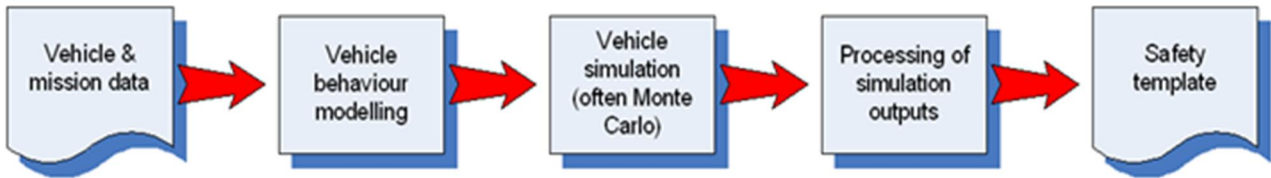
Figure 1. Overview of range safety template generation process using RSTT
