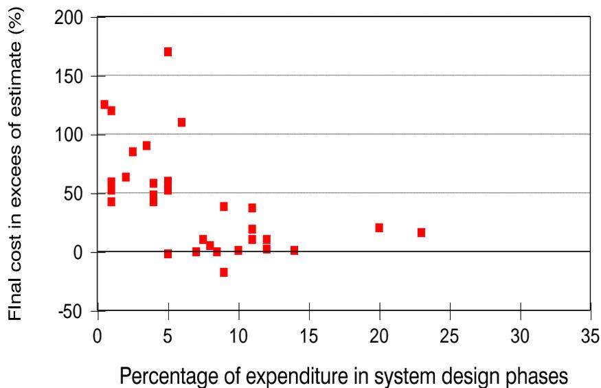
**Figure 1. Cost overrun versus expenditure in systems design phase from NASA (1995).**
