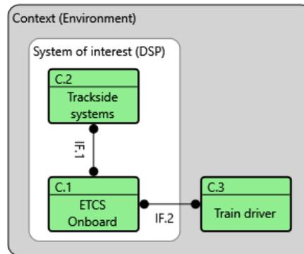
**Figure 8. Example of system interface block diagram**
