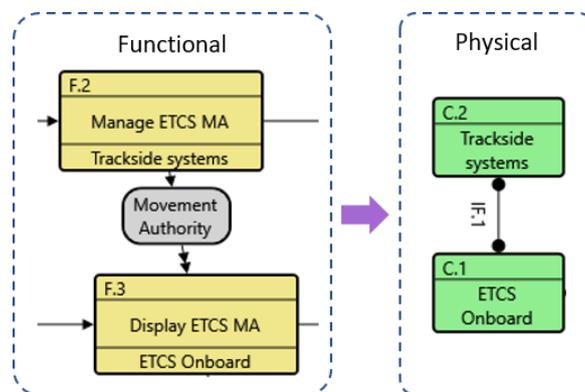
**Figure 7. Example of the derivation of a logical interface from an EFFBD**
